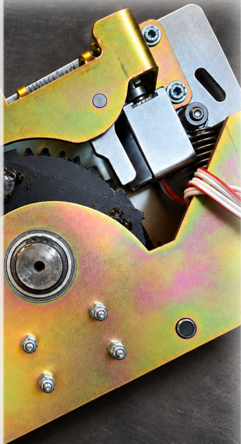
YBT 4132 Single-Lane 4-Arm Turnstile – Internal Mechanism
