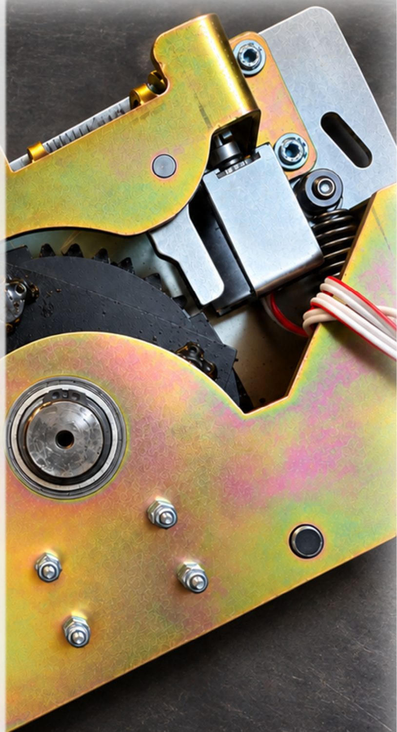
TBT 4145 Single-Lane 4-Arm Turnstile – Internal Mechanism
