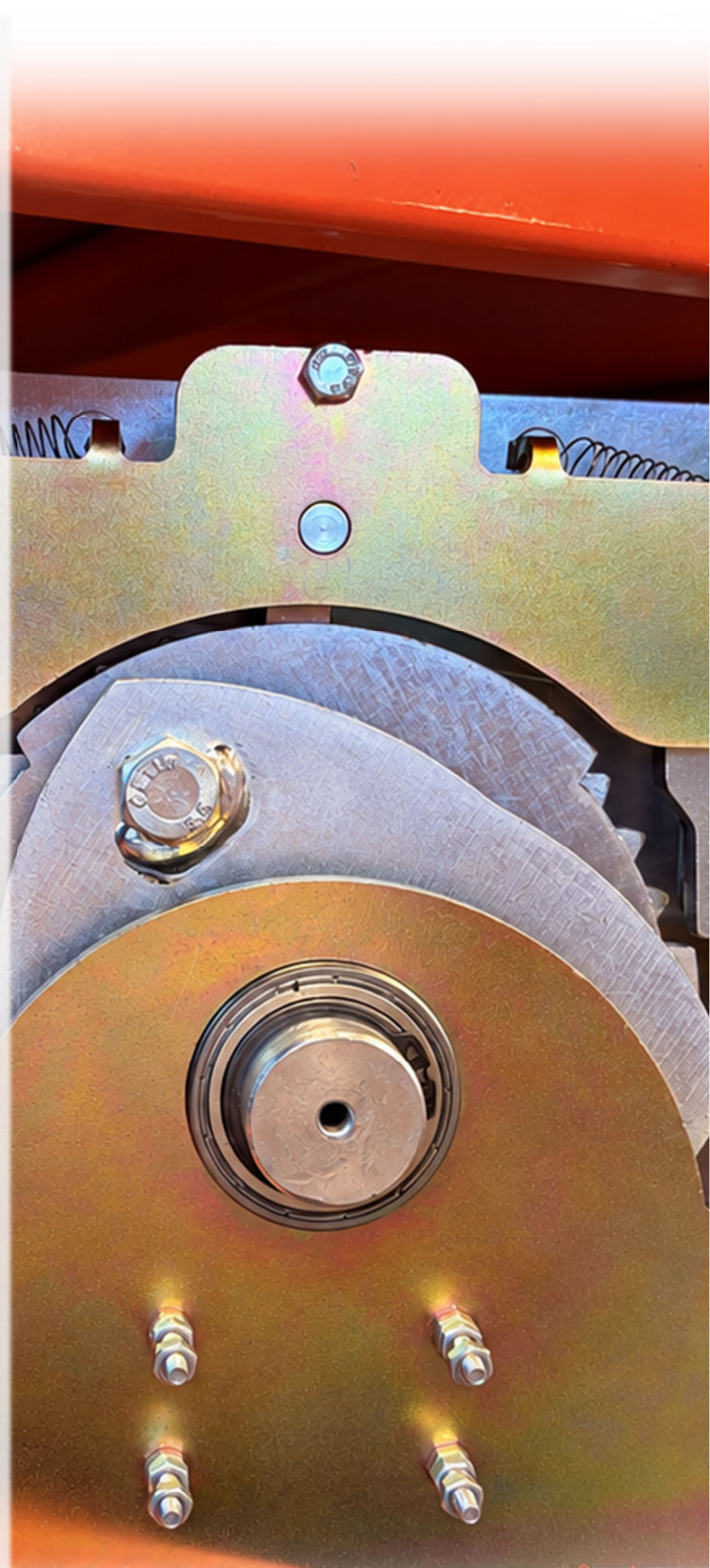
TBT 3220 Double-Lane 3-Arm Turnstile – Internal Mechanism
